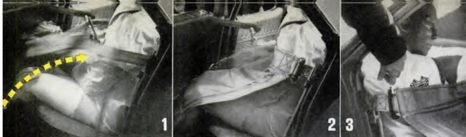
PASSIVE RESTRAINT need not necessarily be the air bag. It can be any device or system that protects drivers and passengers without their having to take any action like buckling a harness. Firestone's research has resulted in a "blanket" system, shown here in a back seat. It snaps into place, pin is pulled for release
